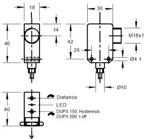
Use the miniature screw driver which is included for adjustment of the two potentiometers.
